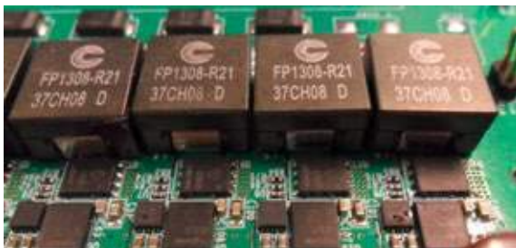
Example: high performance server (PCB: 8 layer, 70 μm)
